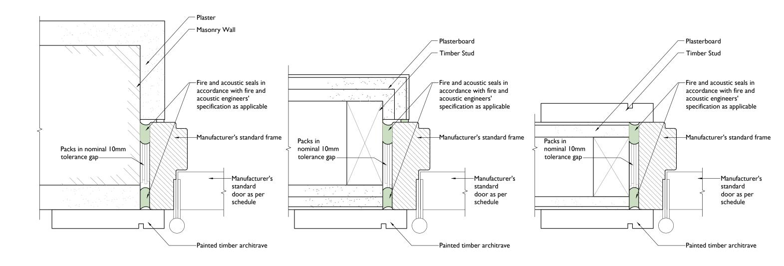
8059-01, Plan: Typical door interface detail with masonry wall Scale: 1:2 8059-02, Plan: Typical door interface detail with timber stud wall Scale: 1:2 8059-03,
