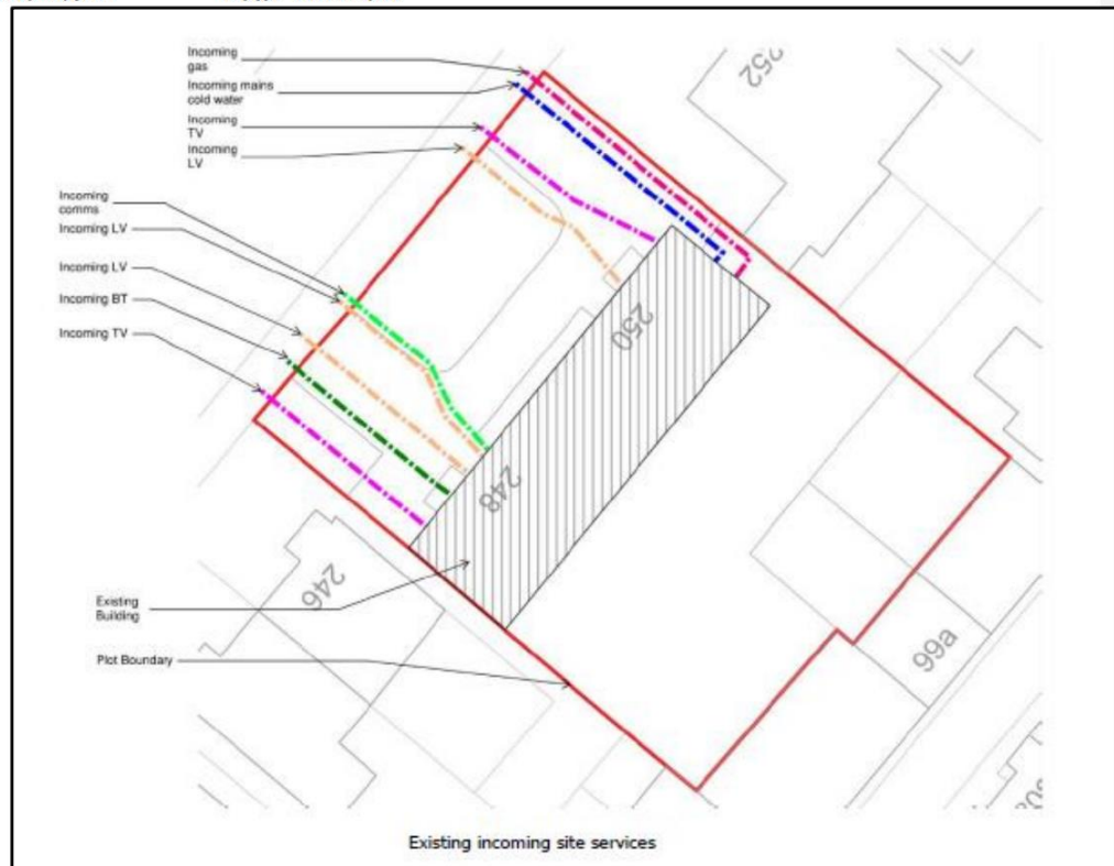
Plan 2 - existing services - from Goody Demolition – Demolition Phase Health and Safety Plan Revision 004
