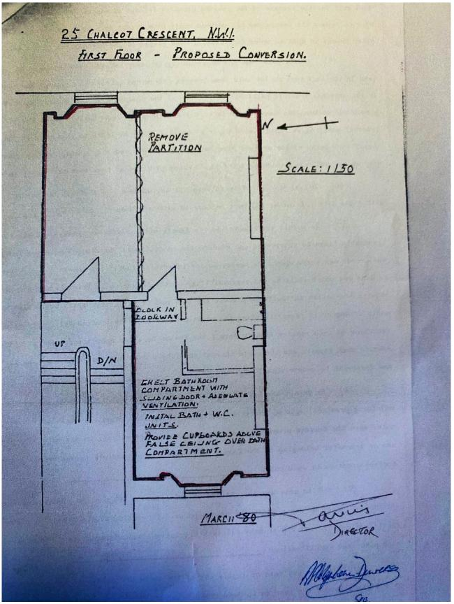
Illustration 2: details of the conversion that took place sometime between March-October 1980, from documents registered at HM Land Registry which reads: "remove partition", "block in doorway" and "erect bathroom compartment with sliding door and adequate ventilation", "install bath and WC units" "provide cupboards above false ceiling over bath compartment".
