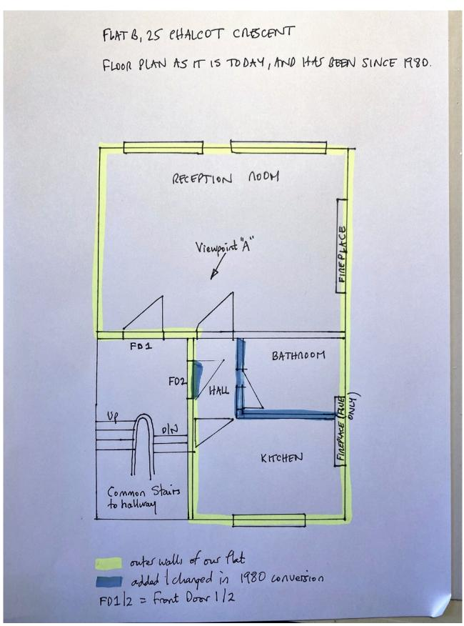
Illustration 1: the layout of the flat as it is today, which has remained unchanged since 1980 and which we do not intend to change (not to scale). Note that the 'fireplace' in the kitchen has only comprised of a boarded-up flue since 1980.
