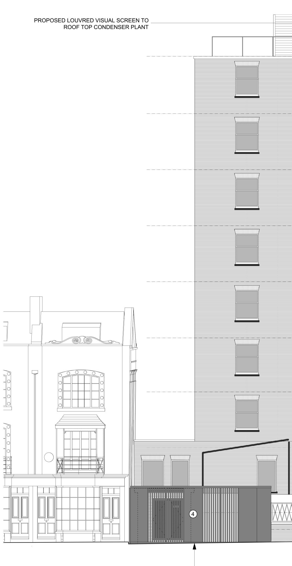
PROPOSED DARK GREY METAL REPLACEMENT BOUNDARY WALL WITH ACCESS TO NEW SUBSTATION BEHIND (DASHED) AND MODIFIED FIRE ESCAPE ACCESS
