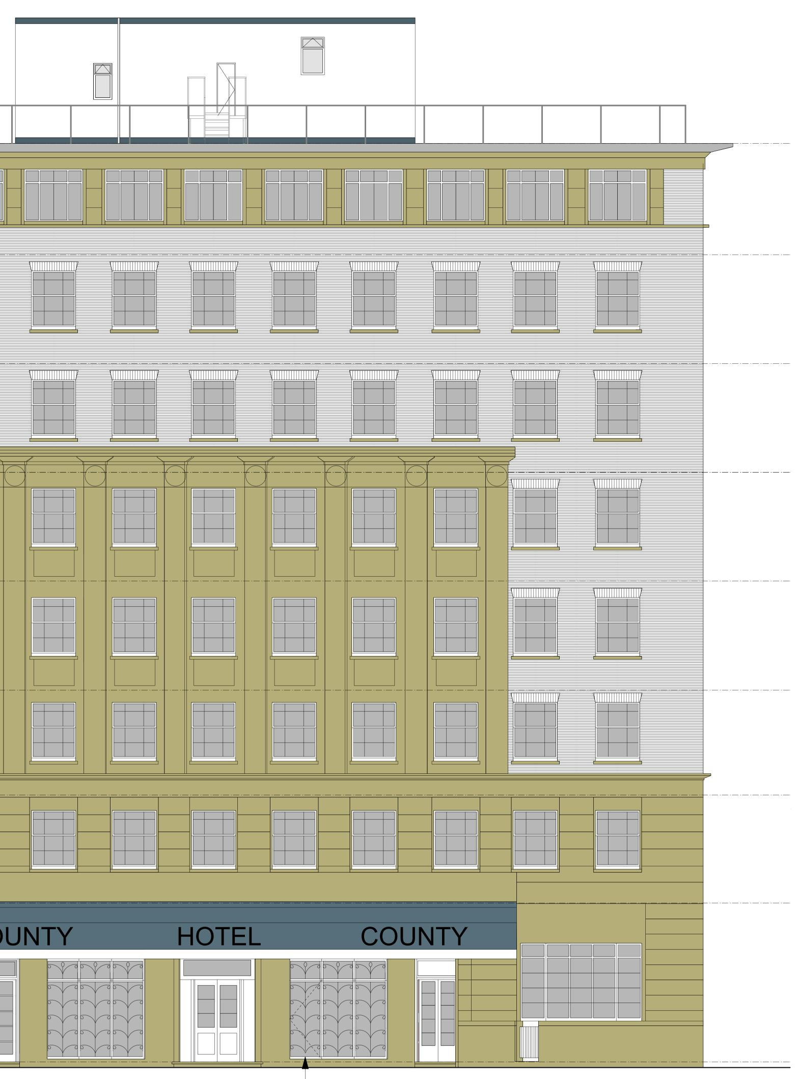
DOOR WIDENED BY 50MM TO ALLOW FOR 850 CLEAR OPENING FOR WHEELCHAIR EGRESS FROM NEW PROPOSED EVACUATION LIFT.
