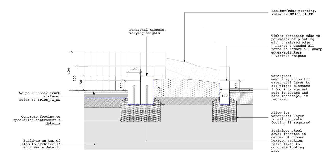
Section 03 - Hexagonal timbers fixing detail
