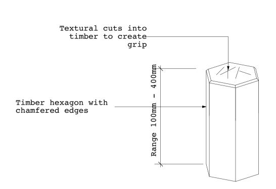
Treated hexagonal timber, varies in height eg.100mm, 150mm, 250mm and 400mm , allow for mix as shown on key plan.
