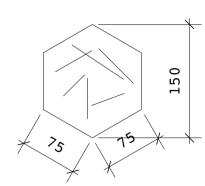
Play garden edge hexagonal timber - type 2: 75mm side width (allow for 135no.)
