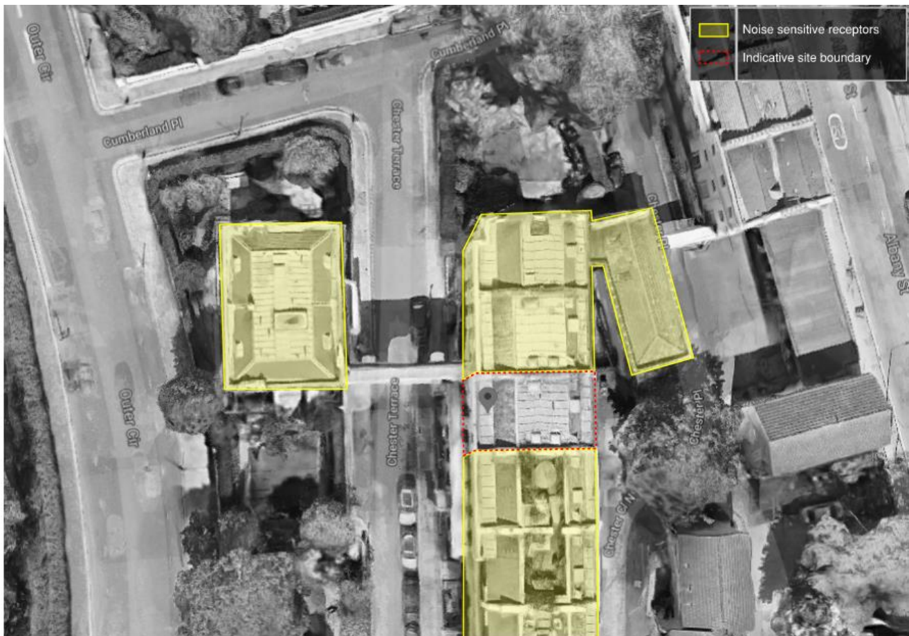
Figure 2-1: Indicative site boundary and nearest noise sensitive receptors (NSR)
