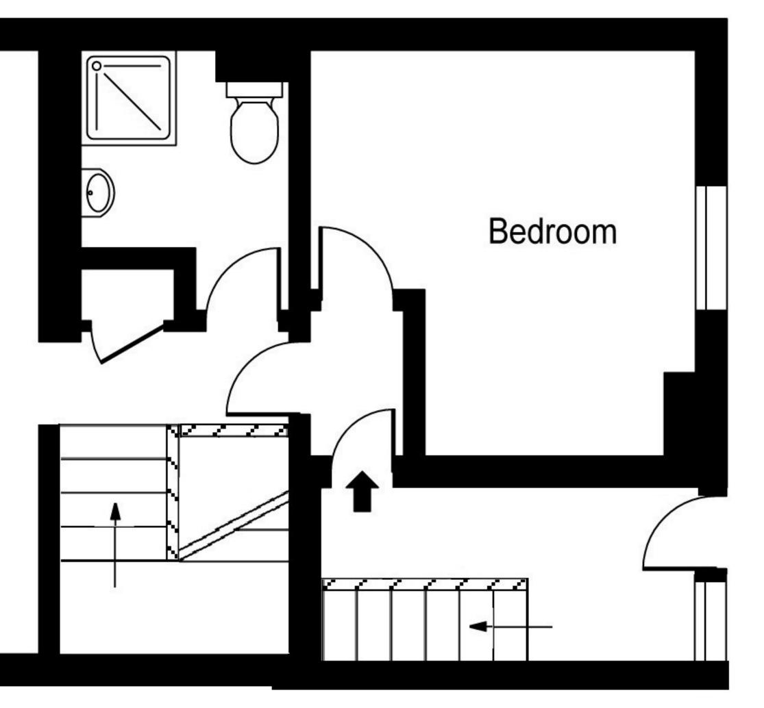
Drawing Title Proposed Floor Plan - Flat C (Raised Ground Floor) Drawing Number P-03 1:50 Scale at A3
