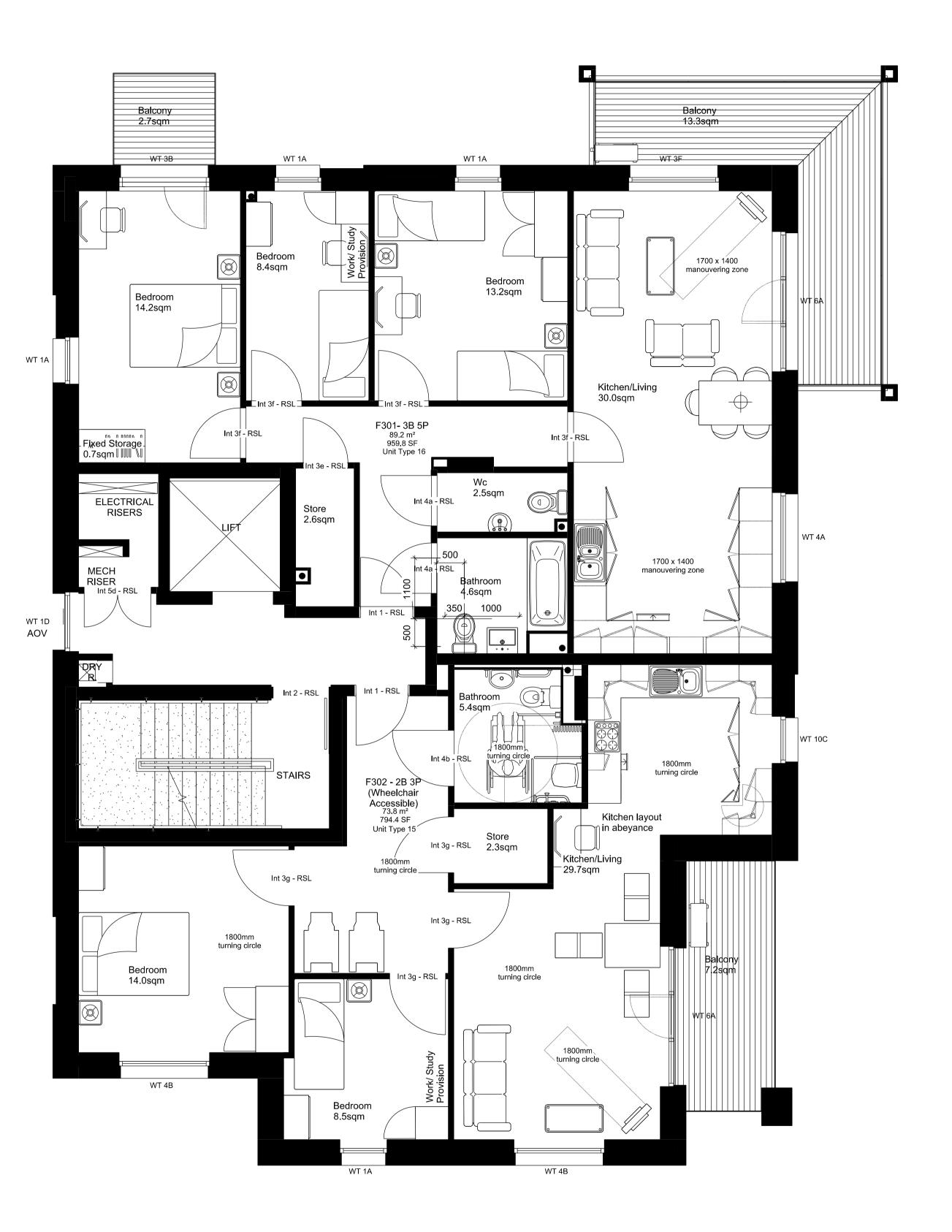
∖Block F - Third Floor Plan 1 - Scale 1:100 at A3
