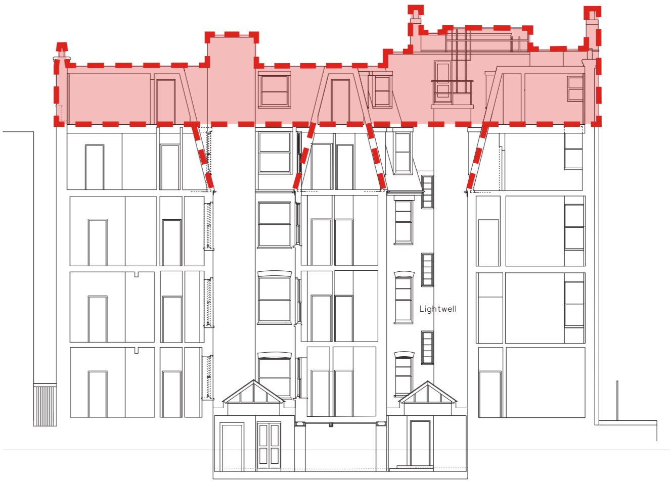
Proposed scheme demolition - Section
