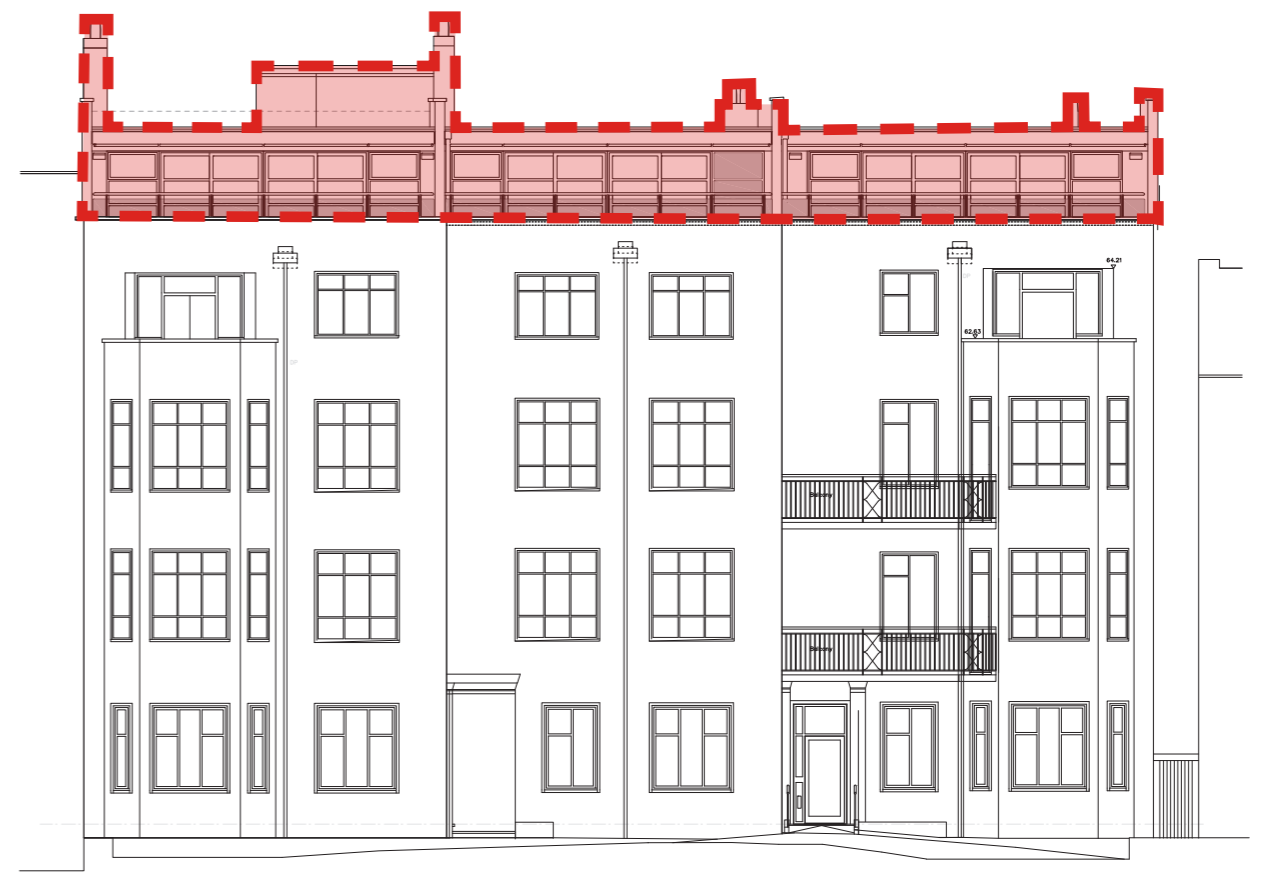
Proposed scheme demolition - Street elevation
