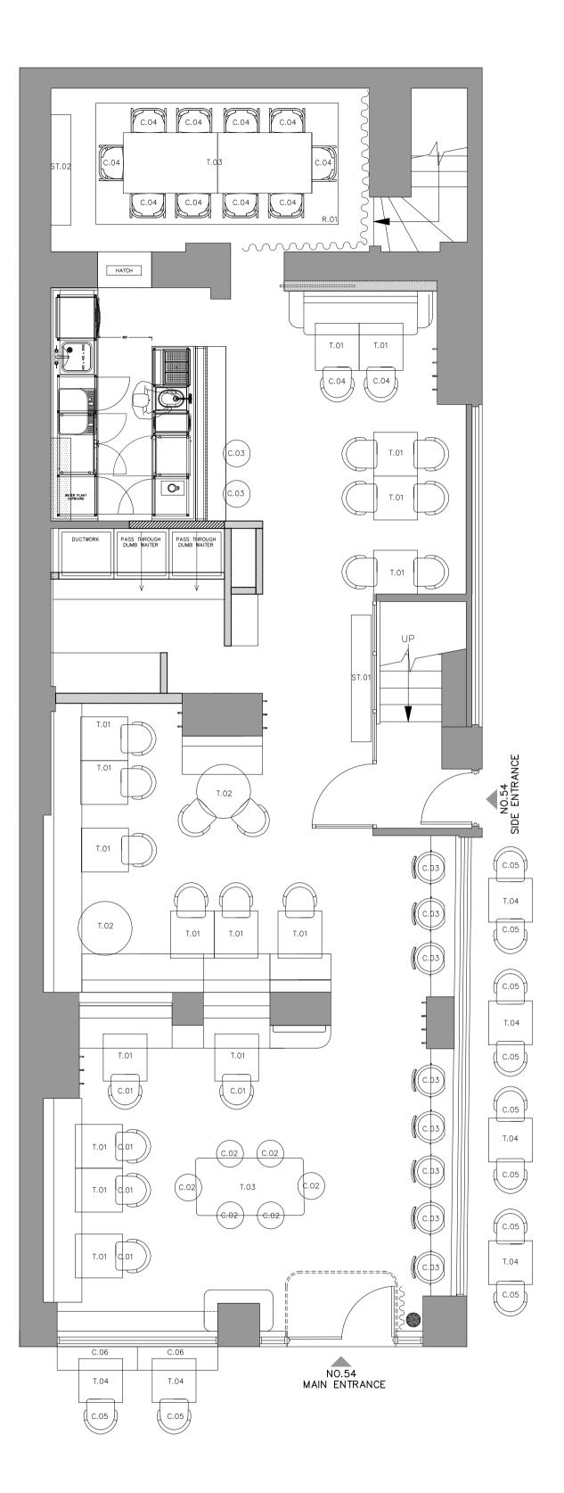
$\bigcirc$  1 ground floor ff&e layout plan 1:50 @ A1
