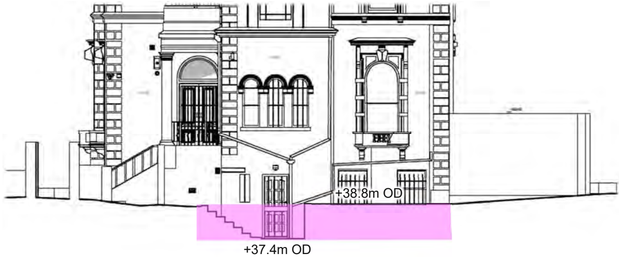
EXISTING SIDE ELEVATION (NORTH) SHOWING PROPOSED EXCAVATION
