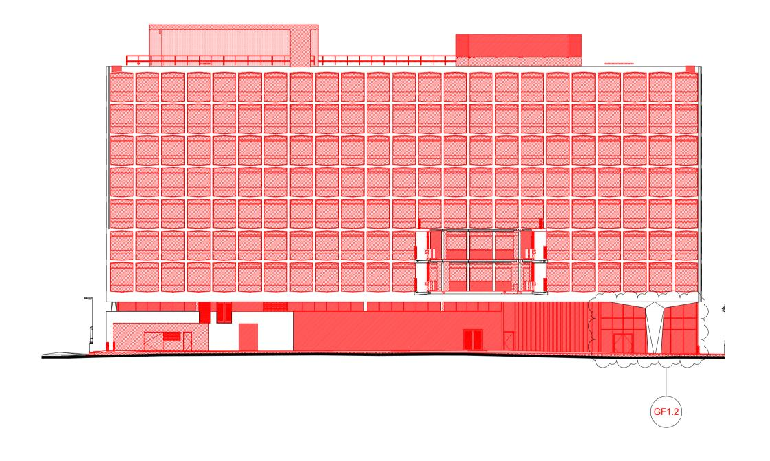
Demolished Structural Elements
