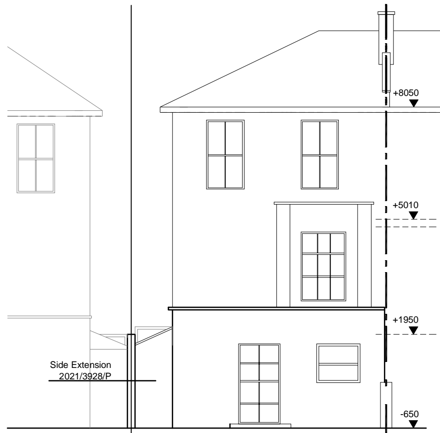
REAR ELEVATION EXISTING SCALE 1:100
