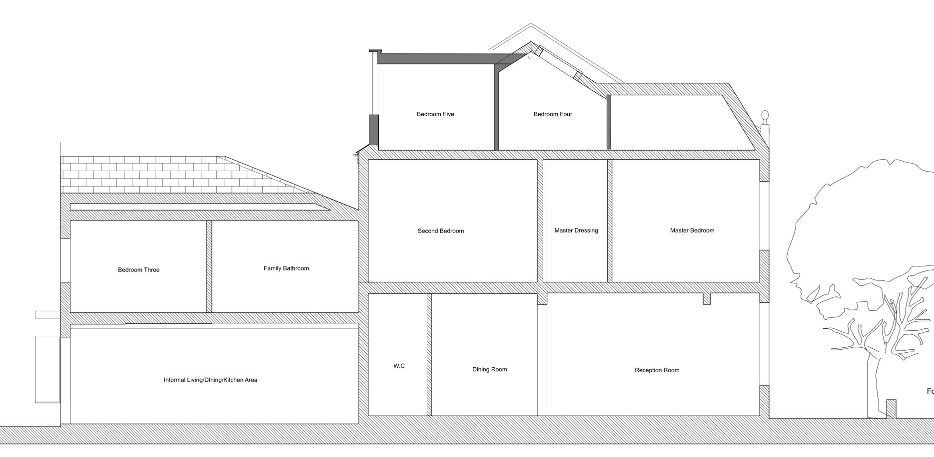
01 Proposed Section AA Scale 1:50@A1, 1:100@A3
