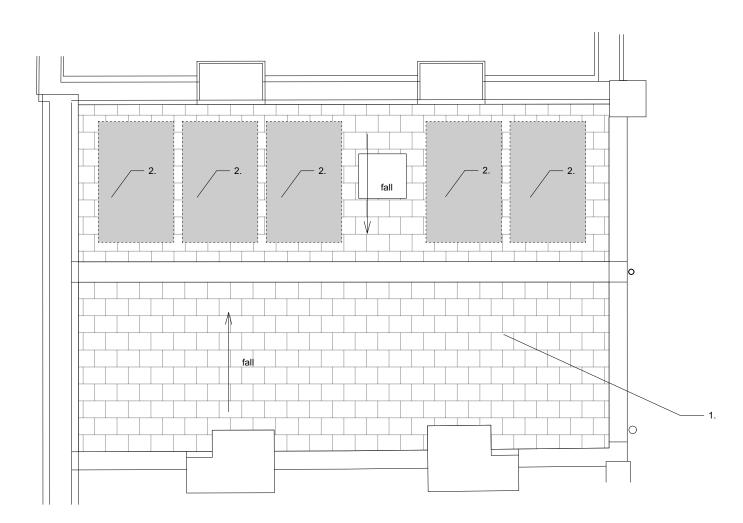
As Proposed Roof Plan Scale: 1:50
