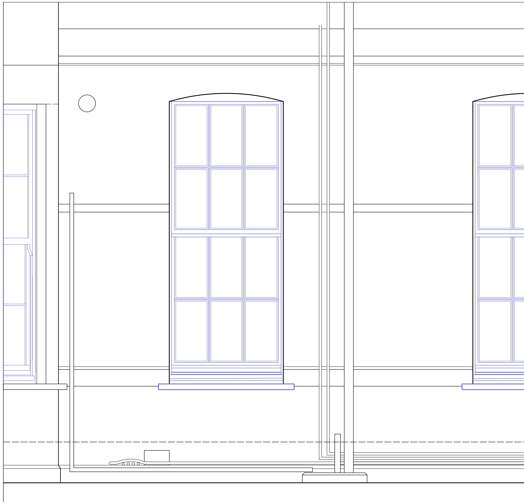
EXISTING ELEVATION OF KITCHEN WINDOW 1:20
