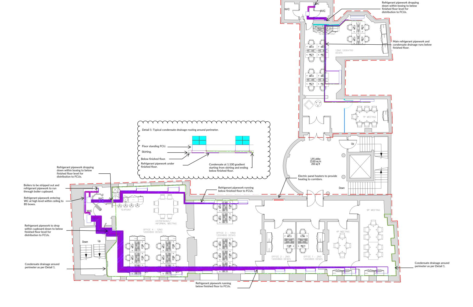
Refrigerant pipework entering WC at high level within ceiling to — BS boxes. Boxing in required to conceal pipework dropping to
