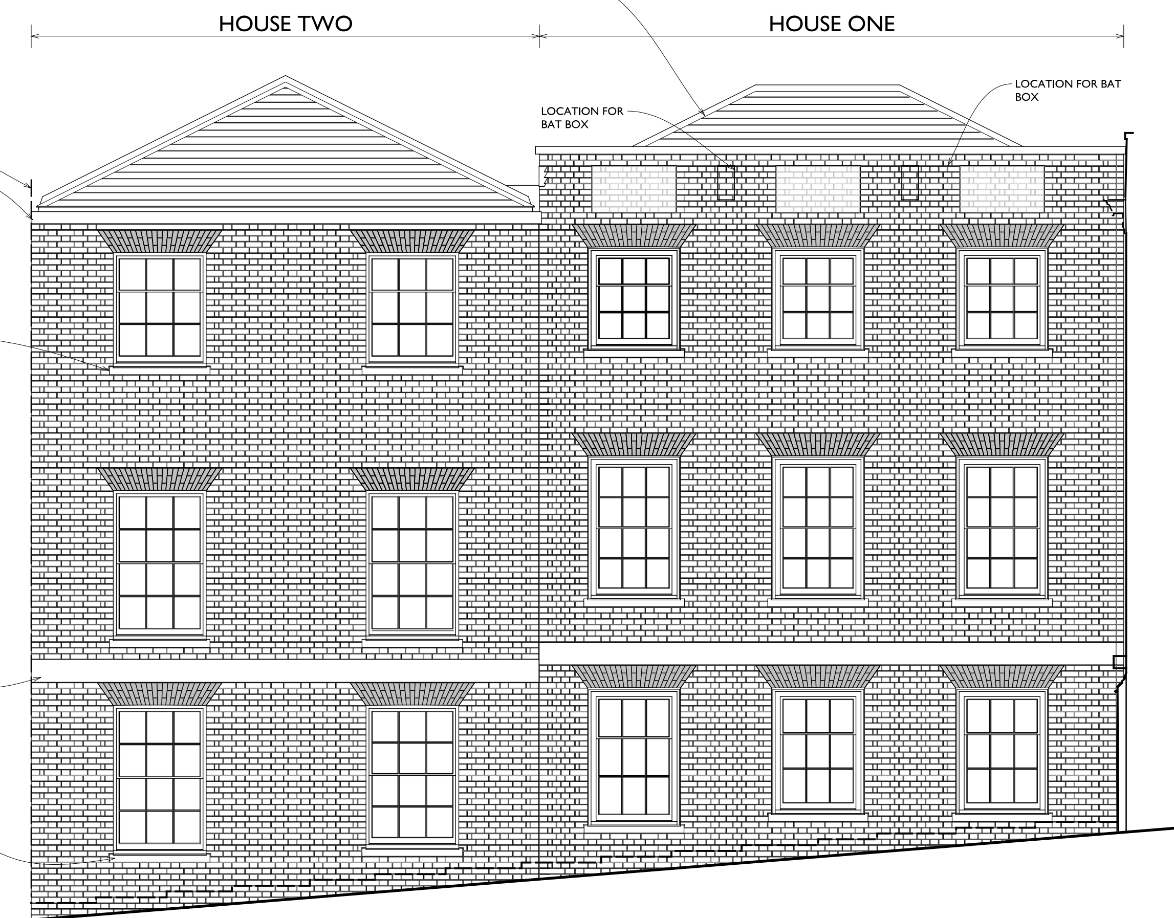
WEST ELEVATION (NO DOWNPIPES TO THIS ELEVATION)
