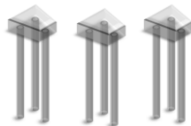
Foundation (piles, pile caps, ground beams) – 17925 tonnes
