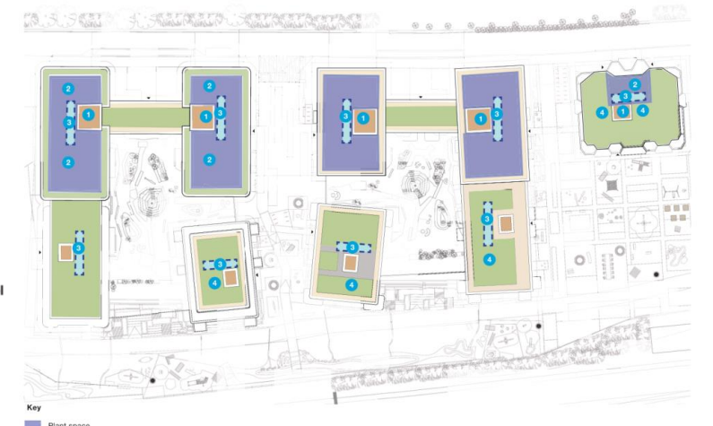
Plant space allocation at Roof Level
