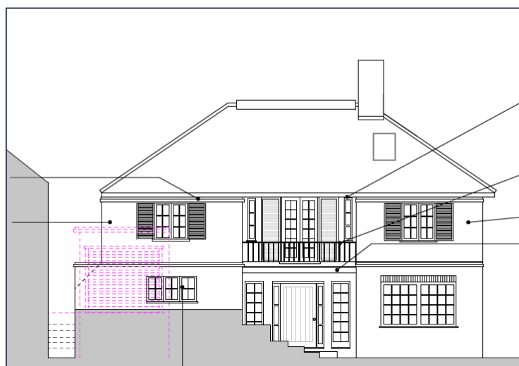
Figure 9- Proposed front elevation (note pink outline shows the existing garage to be replaced)
