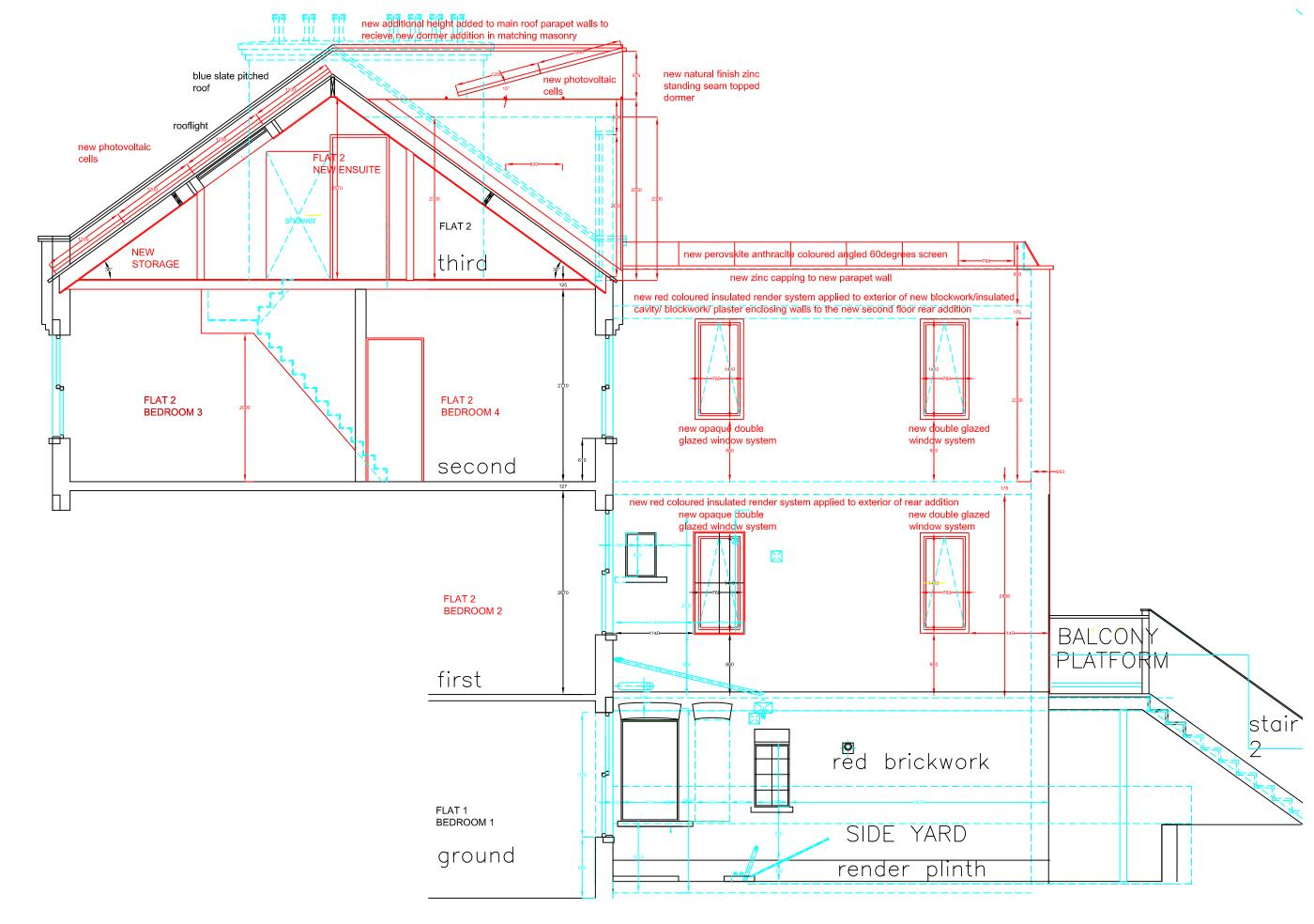
87 CONSTANTINE ROAD, BELSIZE, LONDON NW3 2LP PROPOSED - SECTION B - B & SIDE ELEVATION FLAT 2 © PMRCA P-36 Revision 1
