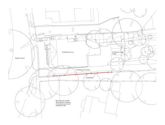
Diagram 02 - Section of the wall to be disassembled and reinstated shown in red
