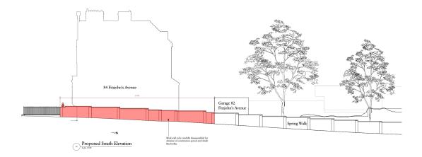
Diagram 01 - Section of the wall to be disassembled and reinstated shown in red
