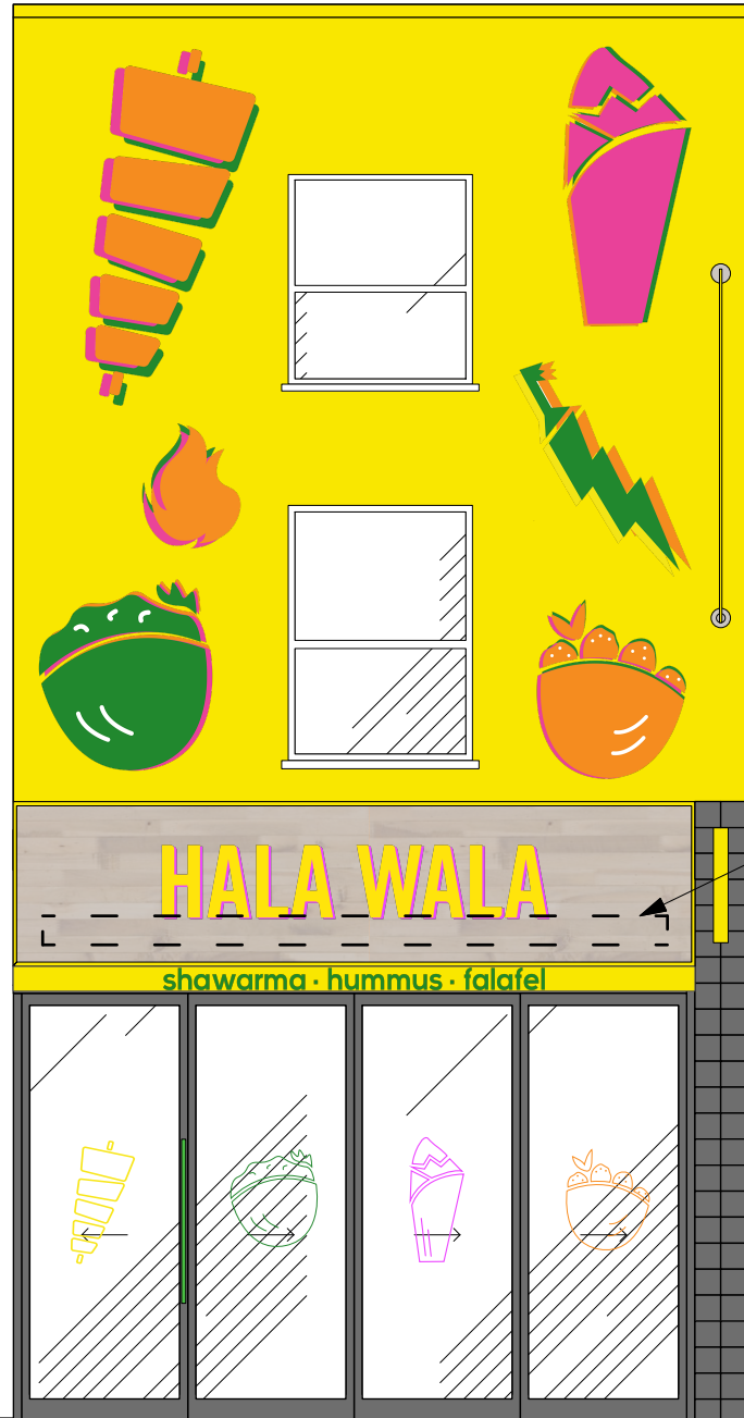
6 PROPOSED FRONT ELEVATION - ILLUSTRATING GRILLE BEHIND FASCIA Scale: 1:50
