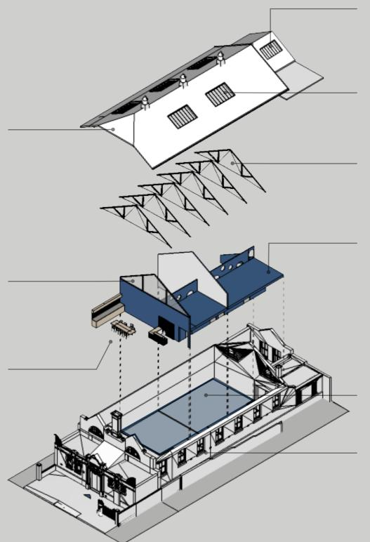
Proposed new double-glazed rooflights to match form and detail of existing rooflights to main hall
