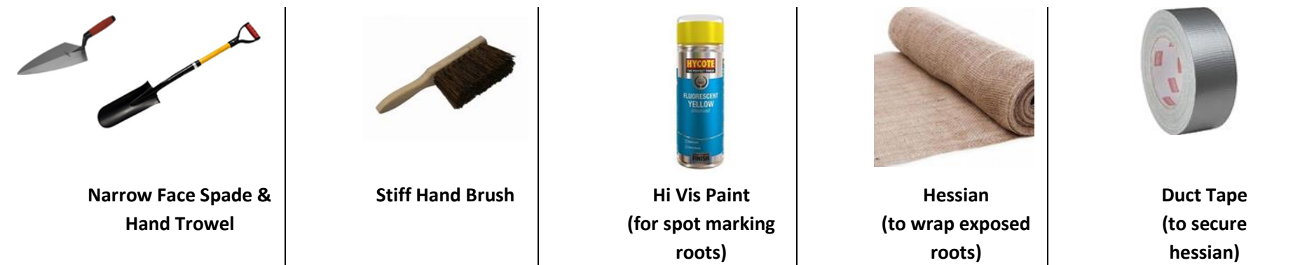
Fig 12 – Advised tools/ materials which should be available for all excavation works within RPA
