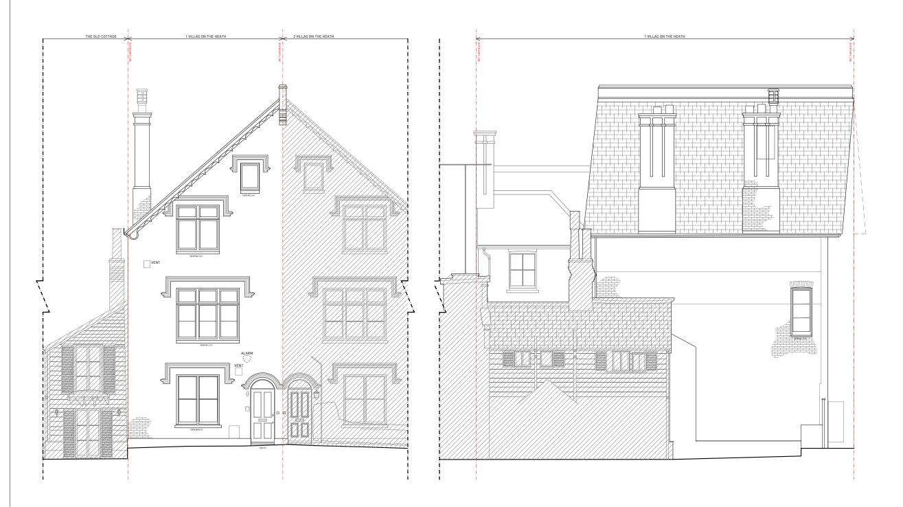
PROPOSED FRONT ELEVATION 1:50 @ A1 / 1:100 @ A3
