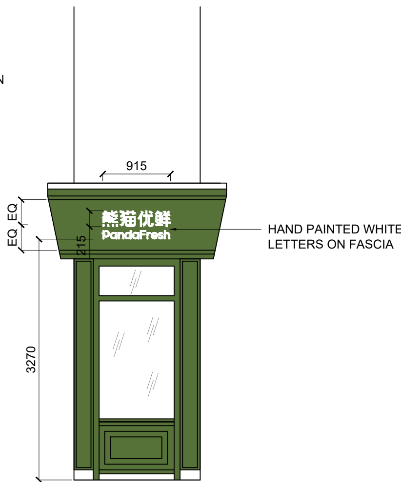
02 SHOPFRONT ELEVATION - CORNER SCALE 1:50 @A1 1:100@ A3
