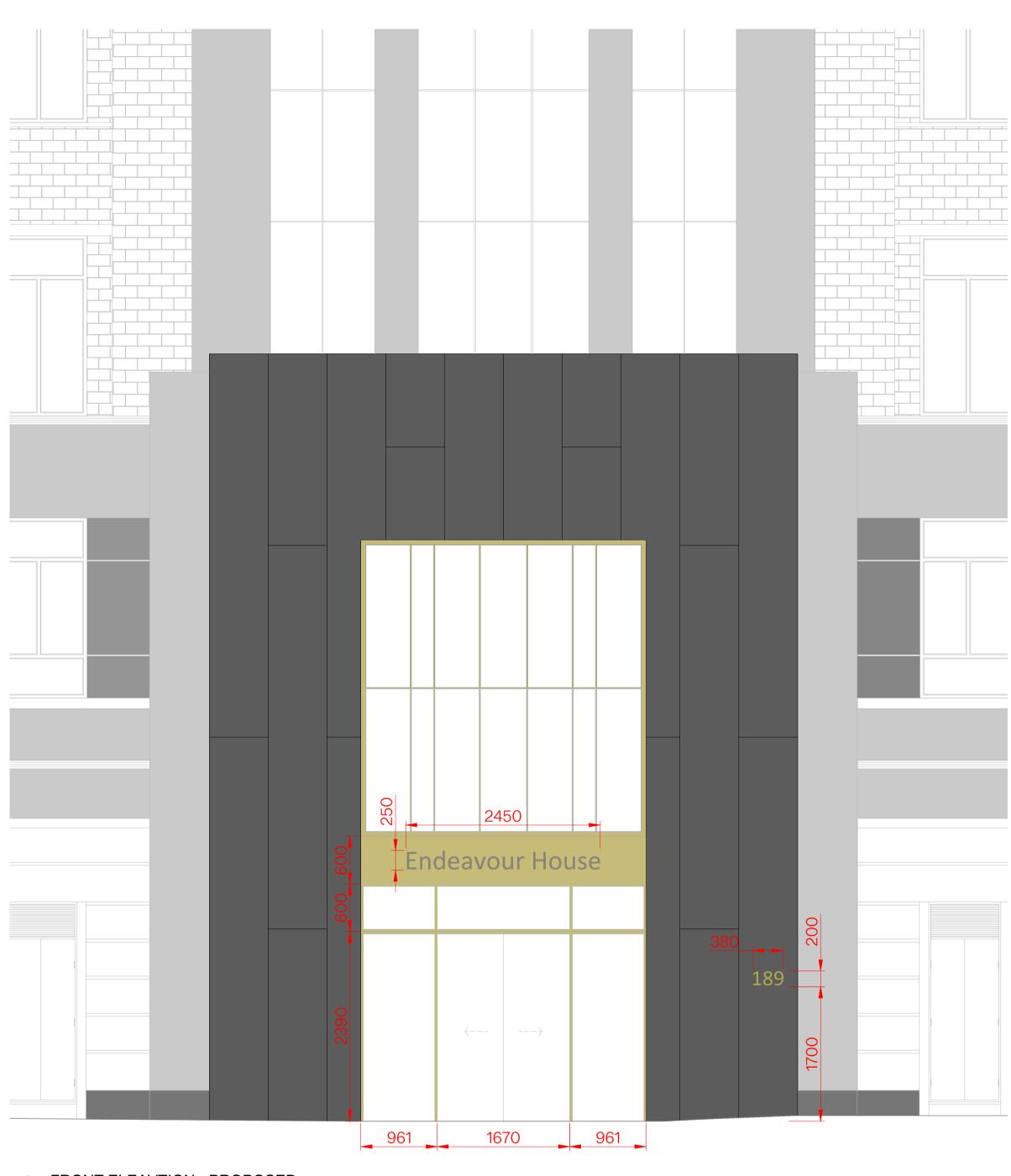
02 FRONT ELEAVTION - PROPOSED Scale: 1:40@A1
