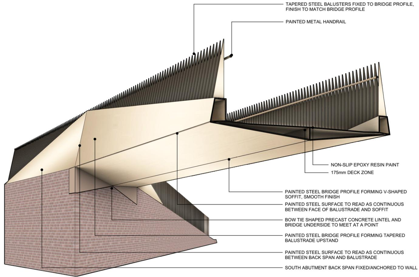
01 SOUTH ABUTMENT SPAN DETAIL 01
