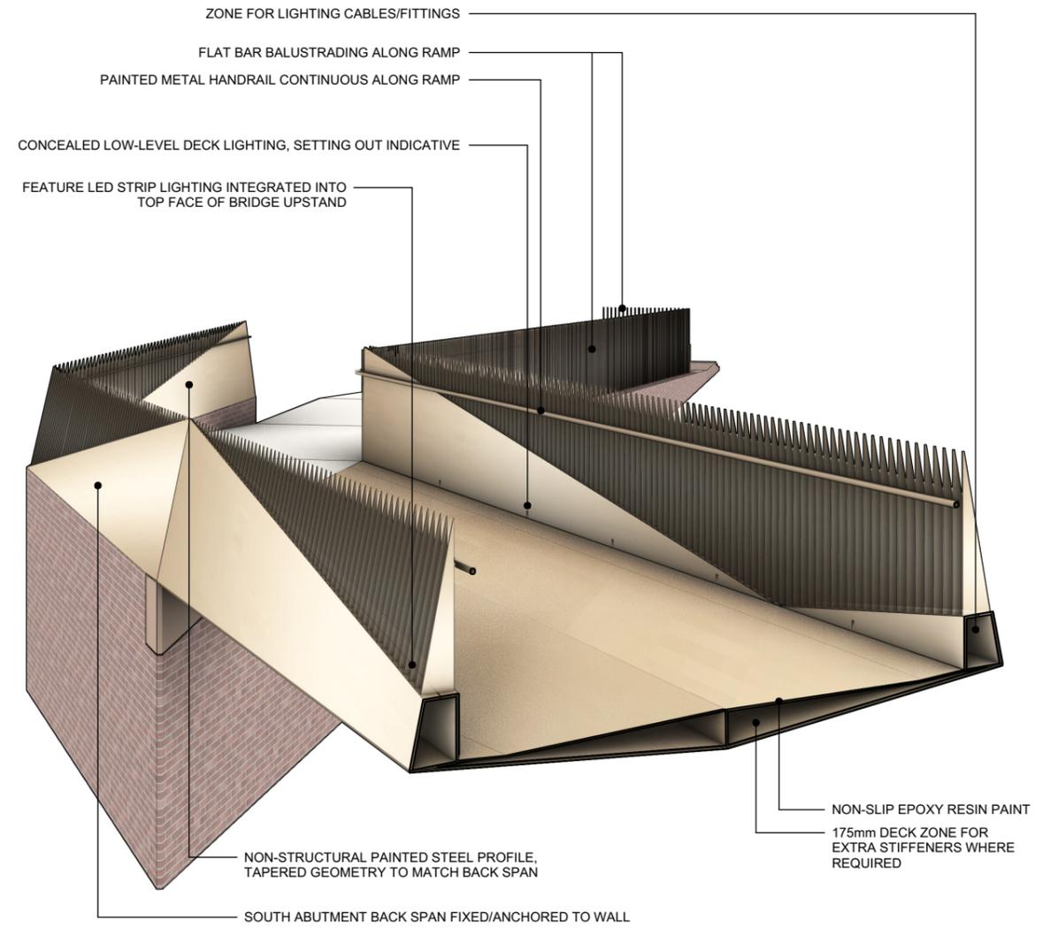
02 SOUTH ABUTMENT SPAN DETAIL 02
