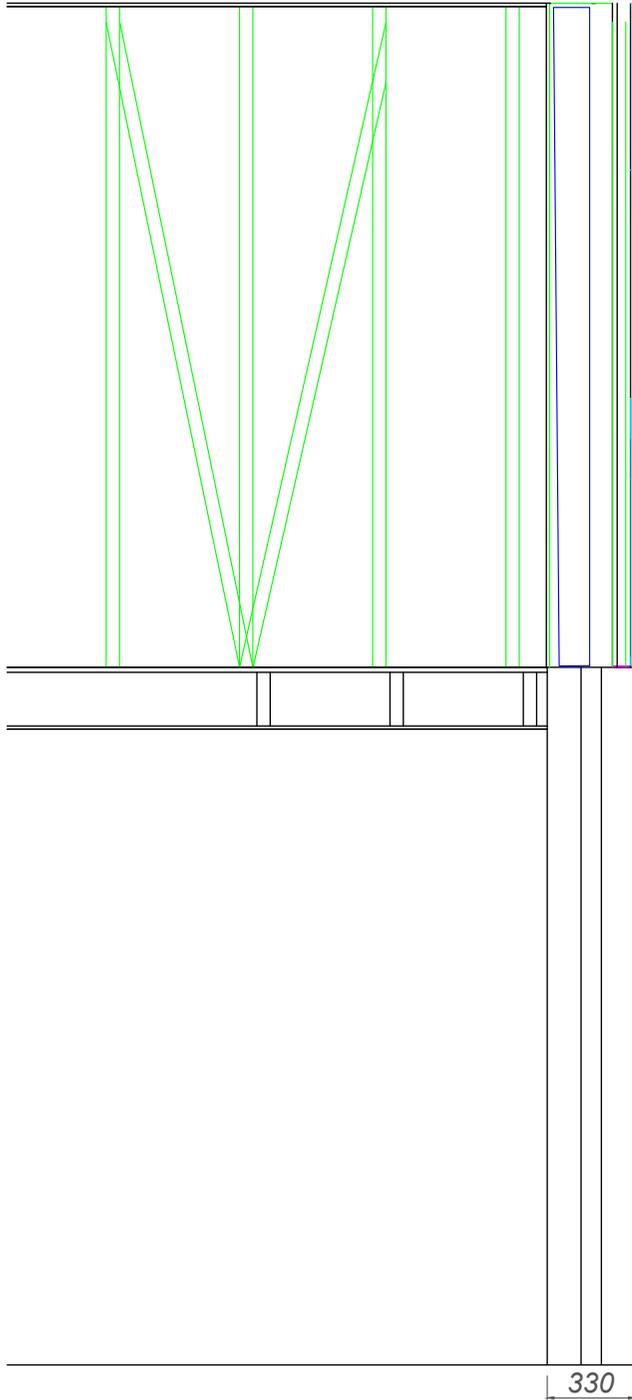
First storey walls - 6 x 2" C16 SW treated wall joists secured into galvanised metal restraint straps at 450mm intervals around perimeter. 6" Celotex insulation between each wall joist. One layer of 12.5 plasterboard screwfixed to interior of stud work wall joists, with joints taped and skimmed over ready for interior decoration.
