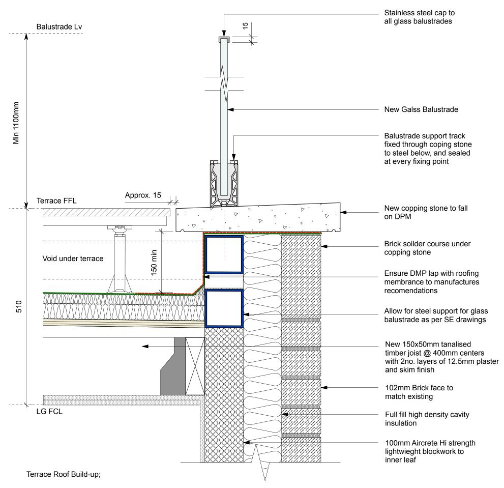
Selected decking boards on rasied pedestal on U-PVC roofing membrance to manufactures recommendations on Kingspan THERMAPROOF TR27 thickness 25mm + 40mm Kingspan OPTIM-R on 18mm WBP plywood on firing piece to fall (Minimun depth 25mm) on min 150mm joist to SE spec and details with 2 no. layers of 12.5mm plasterboard with integral vapour barrier, skim and painted internal finish.
