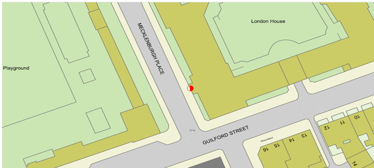
External location for a new 90mm building duct entry to be created into the Lower Ground Comms Room wall from Mecklenburgh Place.
