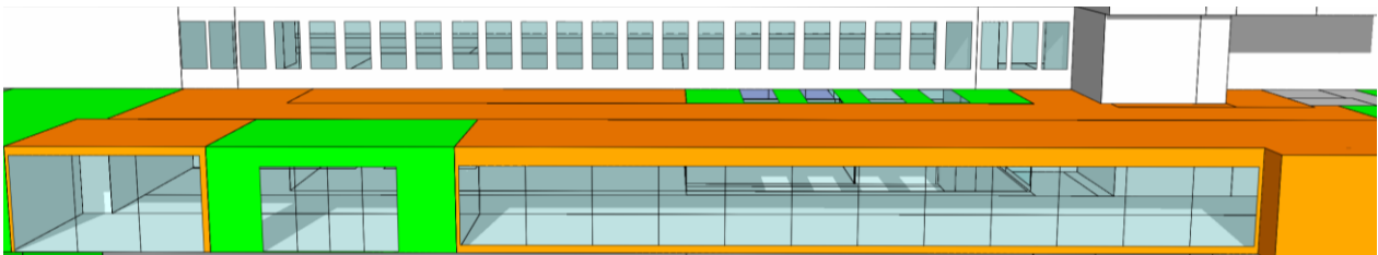
Figure 6—12 Level 4 secondary entrance (green block) and breakout space (orange block) - geometry created in IES
