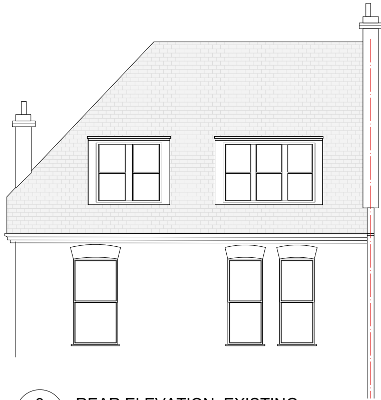
3 REAR ELEVATION_EXISTING SK-05 1:100@A3
