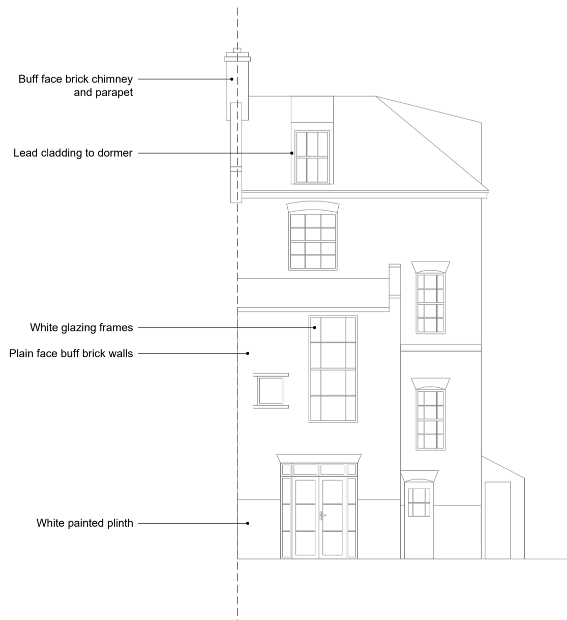
Existing Rear / North Elevation 1/100
