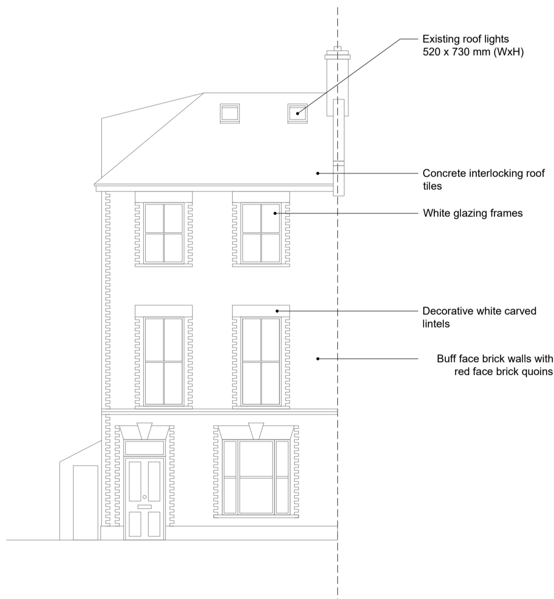
Existing Front / South Elevation 1/100
