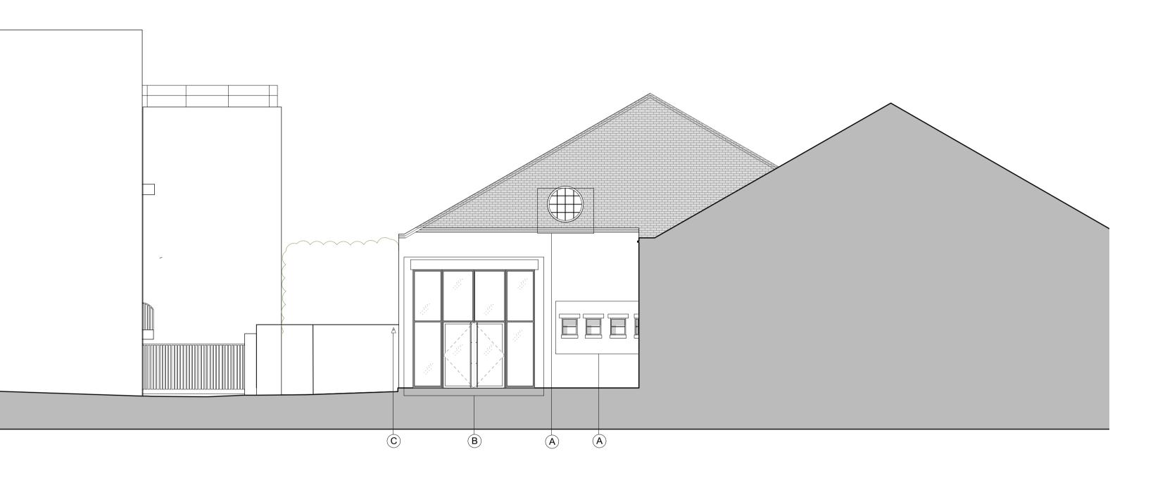
New roof cladding & structure to existing warehouse; to match profile of existing roof F
