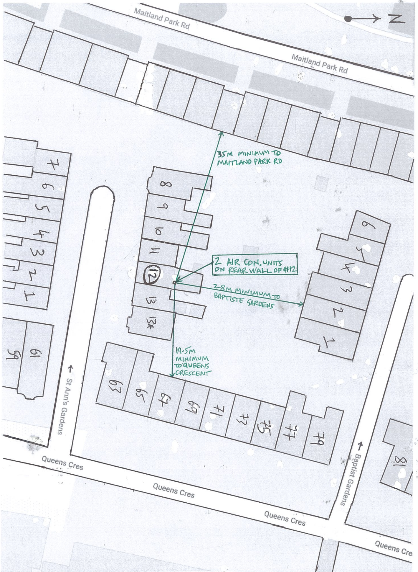
LOCATION PLAN OF #12 ST. ANN'S GARDENS, NWS HER SHOWING PROXIMITY TO NEIGHBOURS OF AIR CONDITIONING UNITS DATE: 27.11.2021 SOURCE: GOOGLE MAPS SCALE: 1:475 DRAWING #: 1 OF 3
