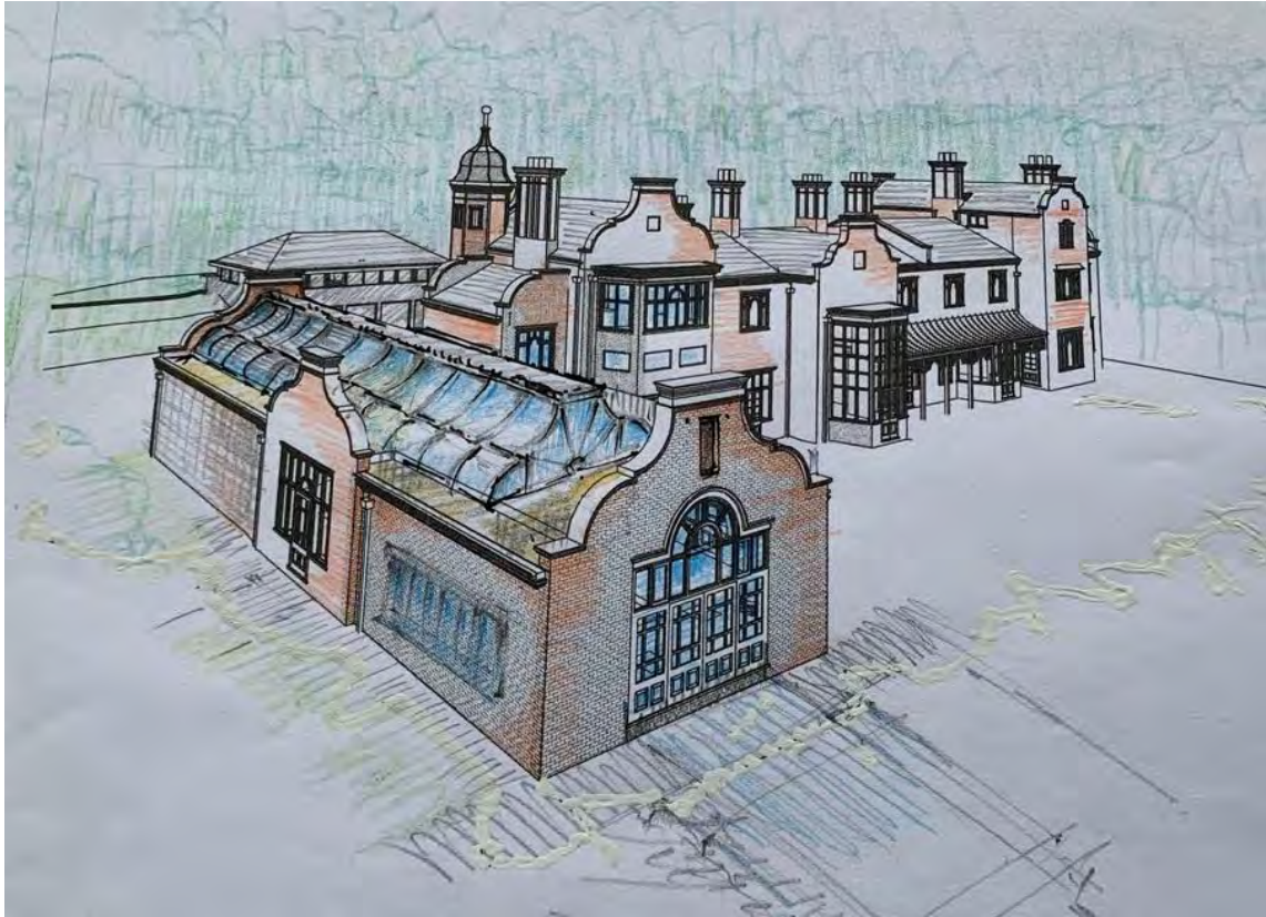
Figure 14 - Early sketch exploring the fully glazed roof – final solution introduced a solid section of the double curved roof
