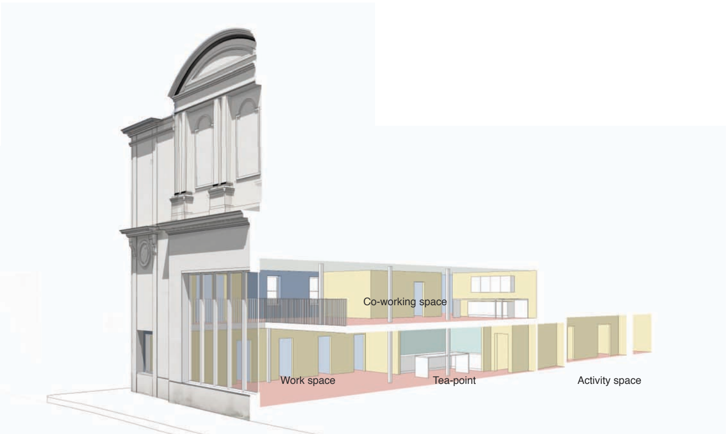
Sectional perspective showing relationship of the new window to the internal accommodation
