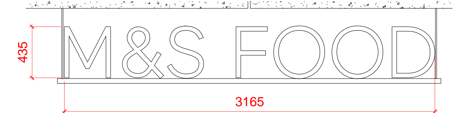
SIGN 3 1 : 20 M&S FOOD LED FACE ILLUMINATED SIGNAGE MOUNTED ON 40MM SHS BAR HUNG FROM SUITBALE POINT IN LINE WITH SE DETAILS
