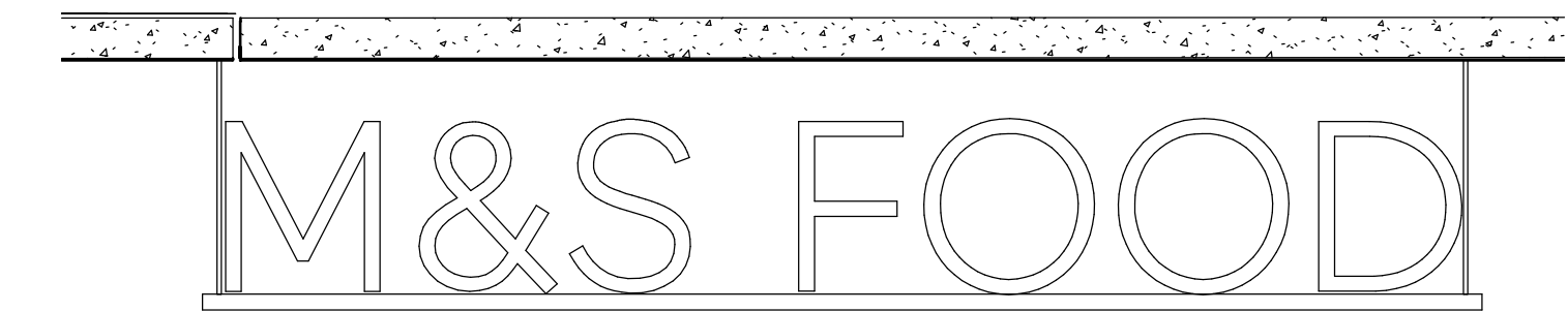
SIGN 1 1 : 20 WHS LED FACE ILLUMINATED SIGNAGE MOUNTED ON 40MM SHS BAR HUNG FROM SUITBALE POINT IN LINE WITH SE DETAILS
