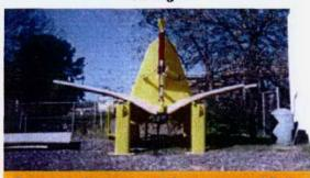
Test apparatus demonstrates mat tolerance to extreme deflection while maintaining high load bearing capacity in pure bending (span = 4 feet (1.2m)). Pure compressive load capacity is approximately 600 psi (40 kg/cm²). Compressive loads in excess of 1000 psi (70 kg/cm²) have been observed in laboratory tests.
