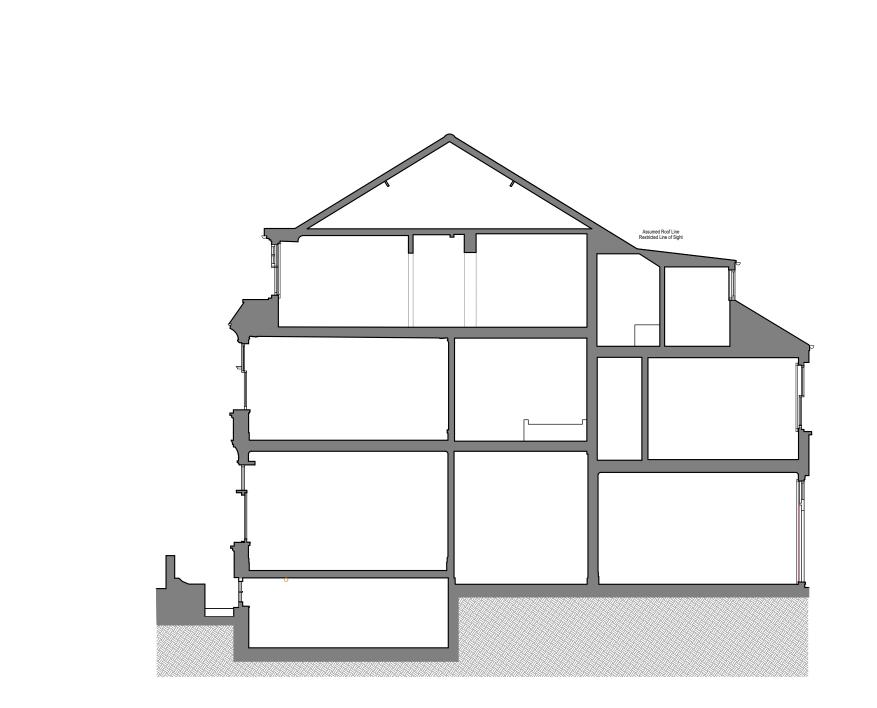
1 SECTION AA AS EXISTING SCALE: 1:100 @ A3 // 1:50 @ A1
