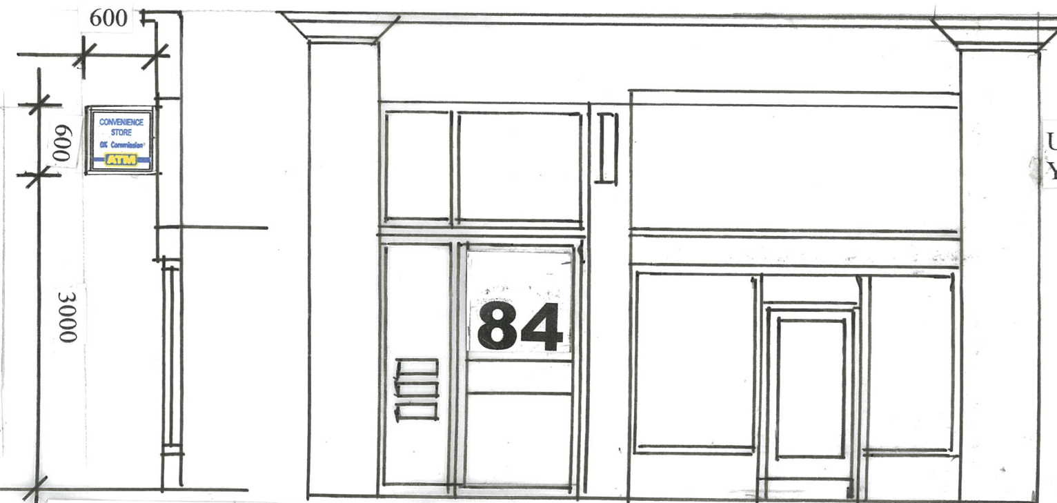
Installed Part Elevation and Section
