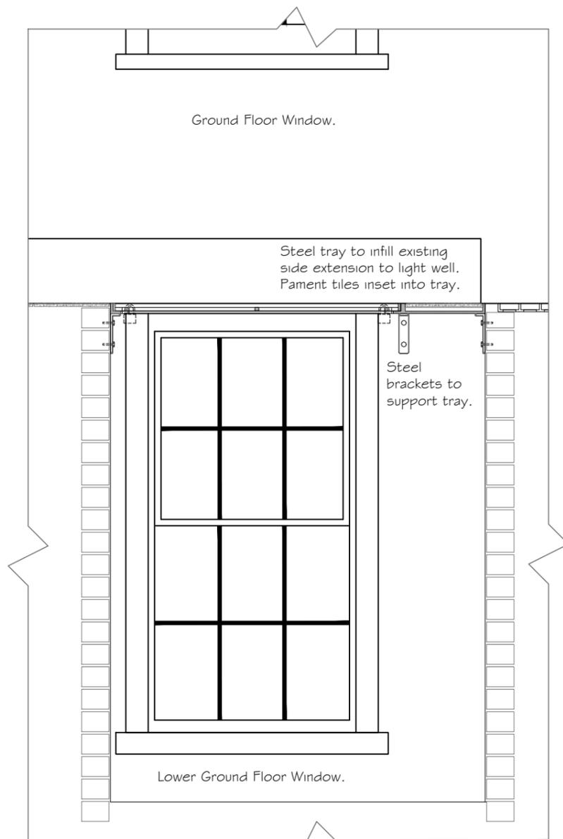
**Proposed Lightwell Grate - Front Elevation.**
