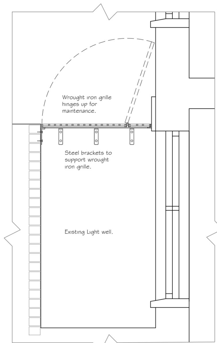
**Proposed Lightwell Grate - Side Elevation.**
