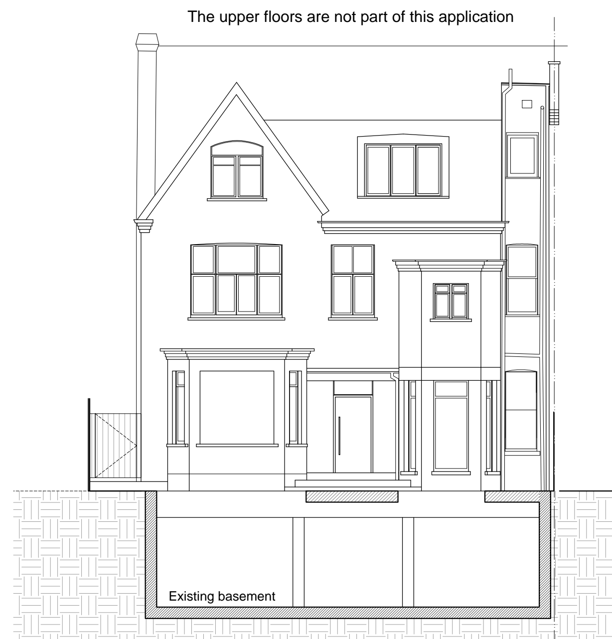
Existing Front Elevation/Section through front lightwell Scale 1:100
