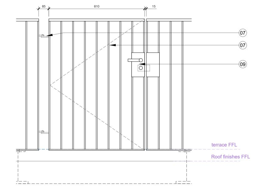
Balustrade Type 1 Typical Elevation and Section 24.607 1:10@A1, 1:20@A3
