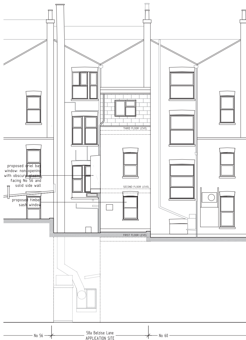
REAR | NORTH WEST | ELEVATION - SECTION A-A
