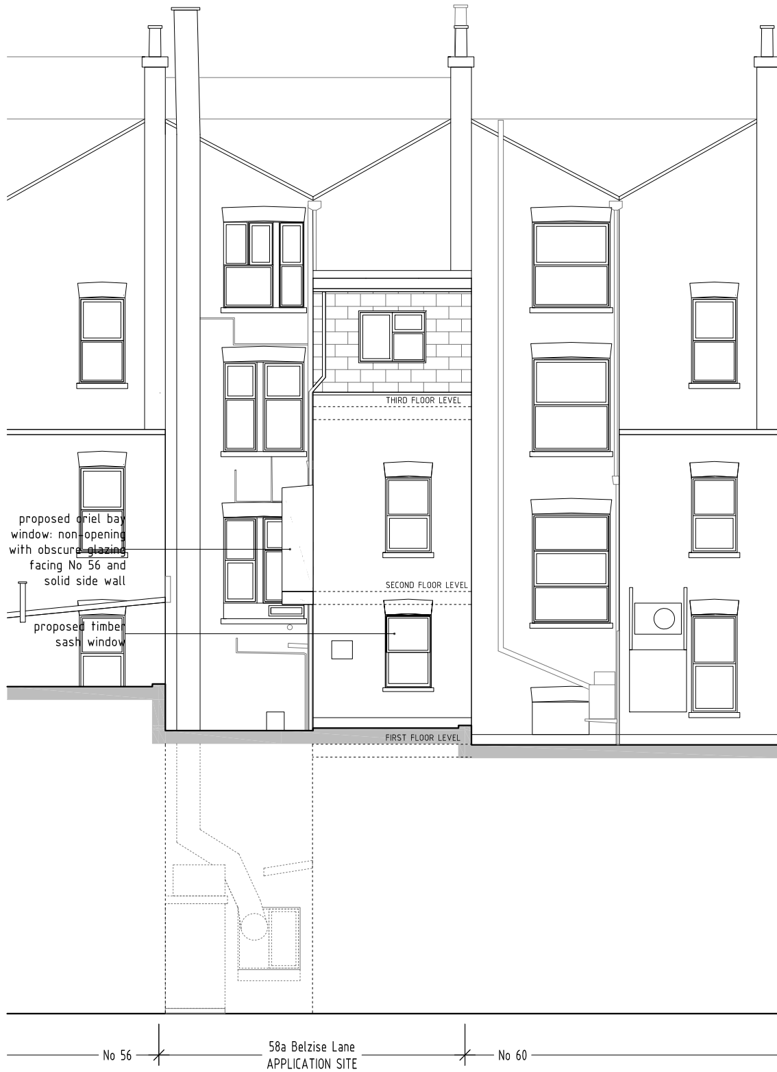
REAR | NORTH WEST | ELEVATION - SECTION A-A
