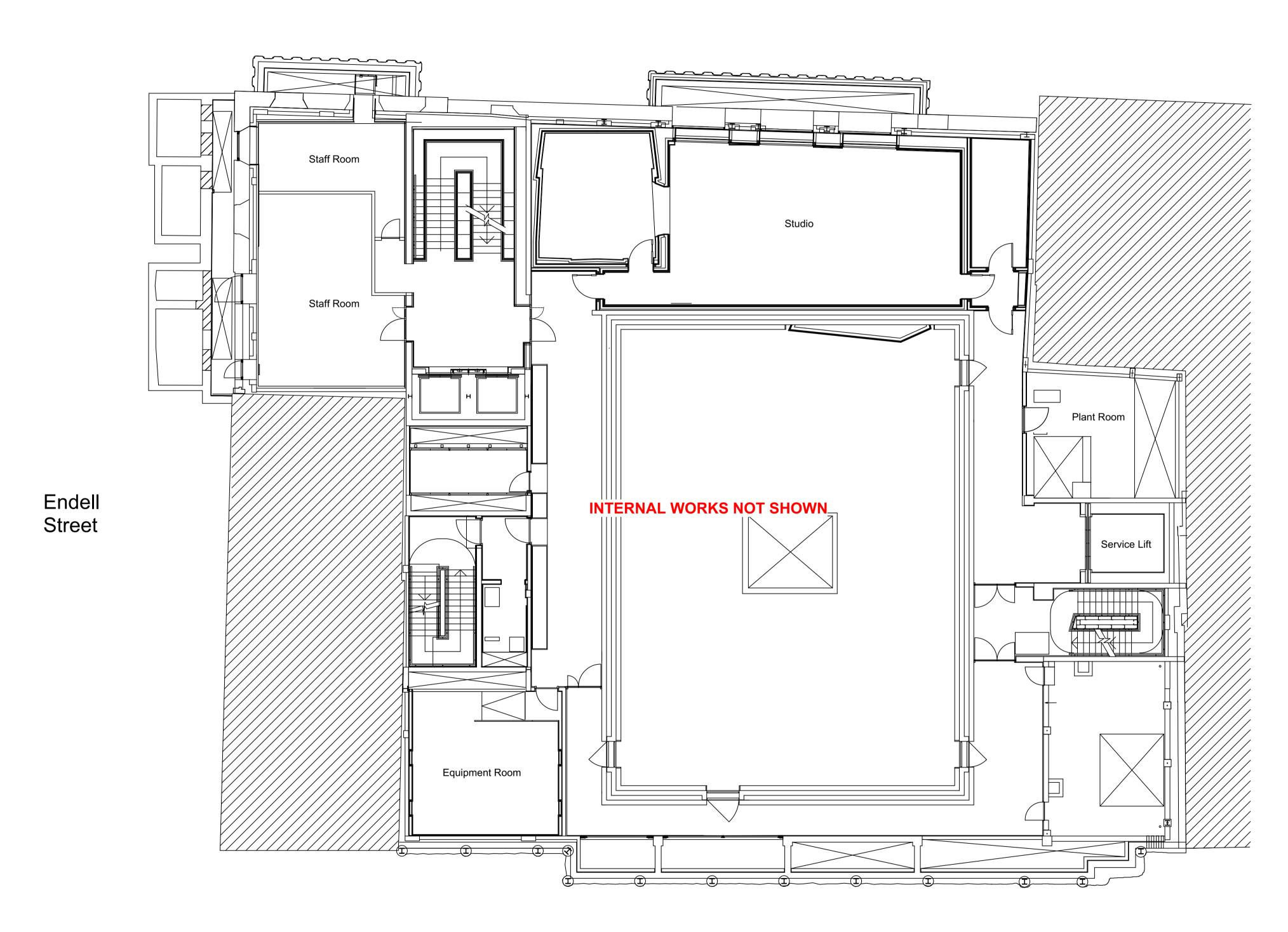
Upper Basement Plan - Demolition Scale: 1:100
